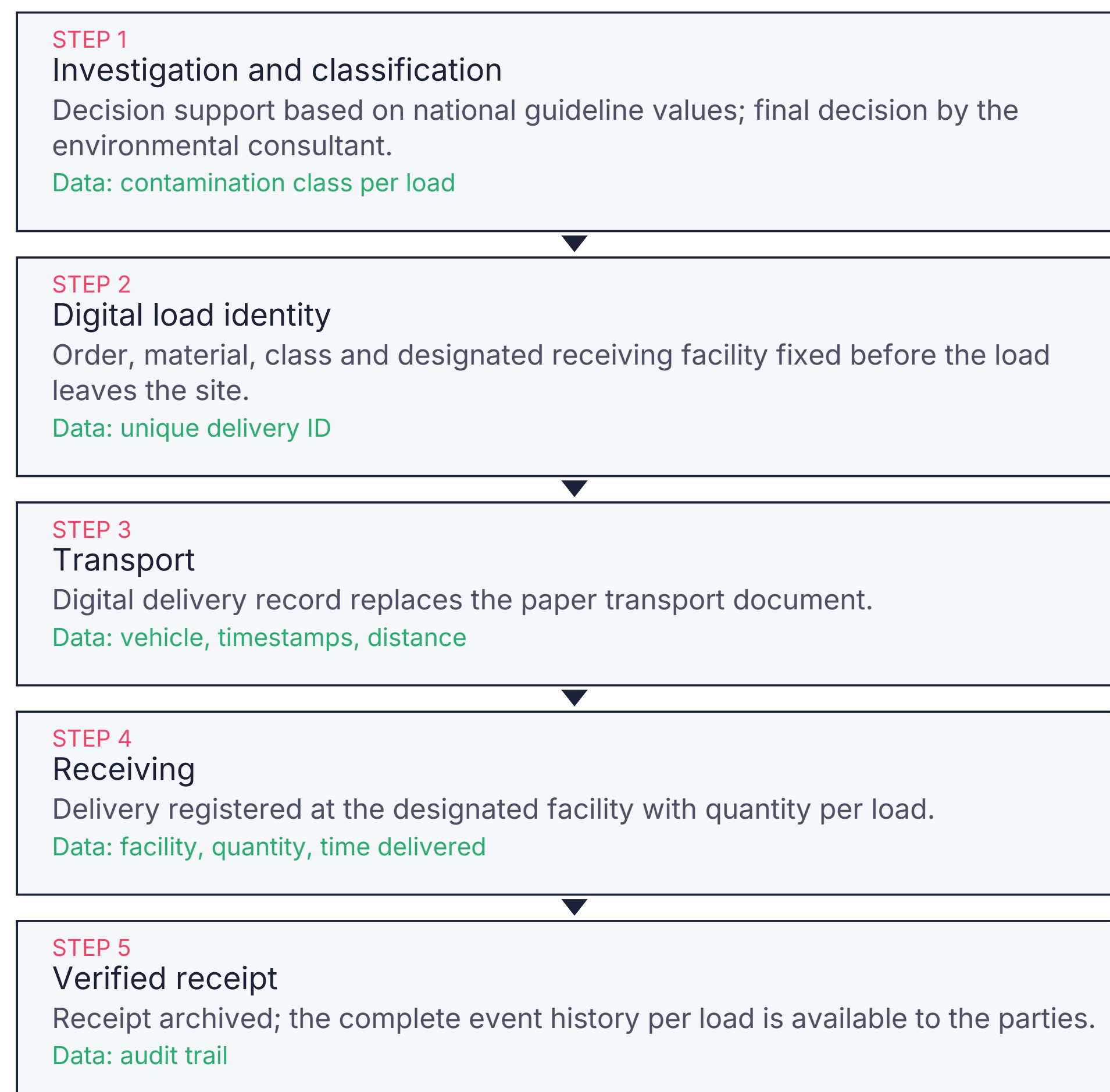
Figure 2. The digital chain-of-custody model as evaluated. Verification data are captured at each step and follow the load through the chain.
